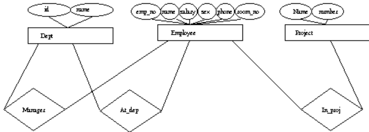
Figure 3.1: Company Entity-Relation Diagram
